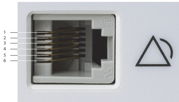
Figure 5-3. Nurse Call Interface Pin Layout
