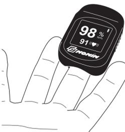
4. View about 4 seconds of readings before relying on the displayed values. Continually verify operation. It is common for the displayed values to vary slightly over a period of several seconds.
